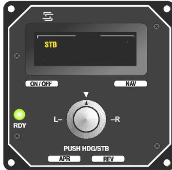
10. ON/OFF Mode Switch engages the roll system in the Stabilizer (STB) Mode. This allows use of the Turn Knob to command up to a standard rate turn. (90%).
