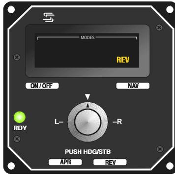
13. Reverse Approach Mode Switch (REV) will engage the Reverse Tracking Mode for use when tracking a localizer back course. This provides APR mode system gain with reverse needle sensing.
