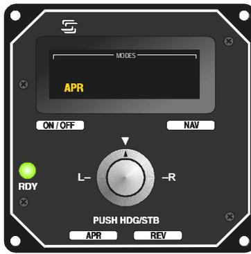
12. Approach Mode Switch (APR) engages the VOR/ GPS/LORAN or Localizer Tracking Mode. This provides a higher level of system gain for more active tracking of VOR, GPS or Localizer front course signals.
