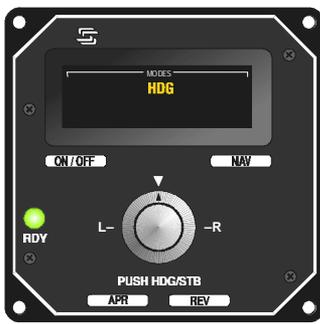
15. To engage the Heading Mode (HDG) if optional DG or HSI is installed, press and release the Turn Knob. To return to STB Mode, press and release the Turn Knob again. When the system is in a NAV mode and there is a DG or HSI installed, press and release the Turn Knob to return to the HDG Mode.
