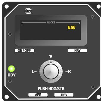
11. Navigation Mode Switch (NAV) will engage the VOR/ GPS/LORAN Tracking Mode. This provides low system gain for comfortable cross-country tracking.
