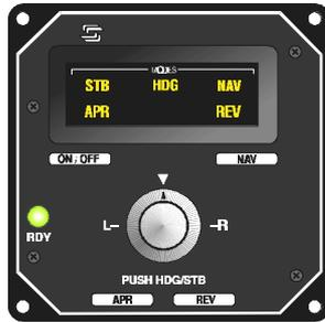
**Note:** The Aircraft (AC) instrument light rheostat controls the annunciator and indicator brightness.
